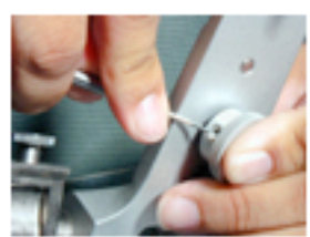
Remove sealing compound covering Hex Screw
