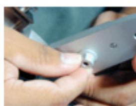
Lightly tighten QuickMount Plate Holder Nut and repeat steps for Lower Member
