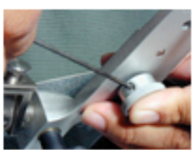
Using Hex Driver, loosen screw
