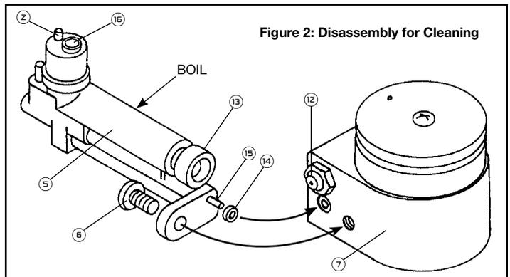
⑭ does not have to be removed, but be careful not to lose it. Use care to not bend the Pilot Inlet Tube ⑮. Before reattaching the Burner Assembly, blow out all water from the Pilot Inlet Tube, Air-Intake Adjustment ⑬, Burner Tube ⑯ and the Pilot Light ②. Make sure that the “O” Ring for the Pilot Inlet Tube is replaced if it was removed.
