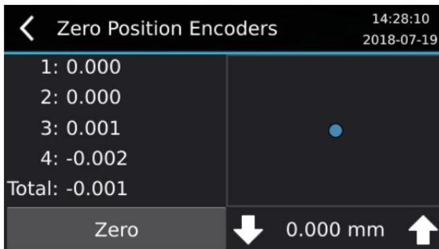
THE ENCODERS 1-4 CAN SHOW NON 0.000 VALUES DUE TO FLUCTUATION (THEY SHOULD FLUCTUATE MAXIMUM BETWEEN +/-0.020). IMPORTANT IS THE TOTAL VALUE. IN THIS EXAMPLE THE TOTAL VALUE IS IN TOLERANCE.
