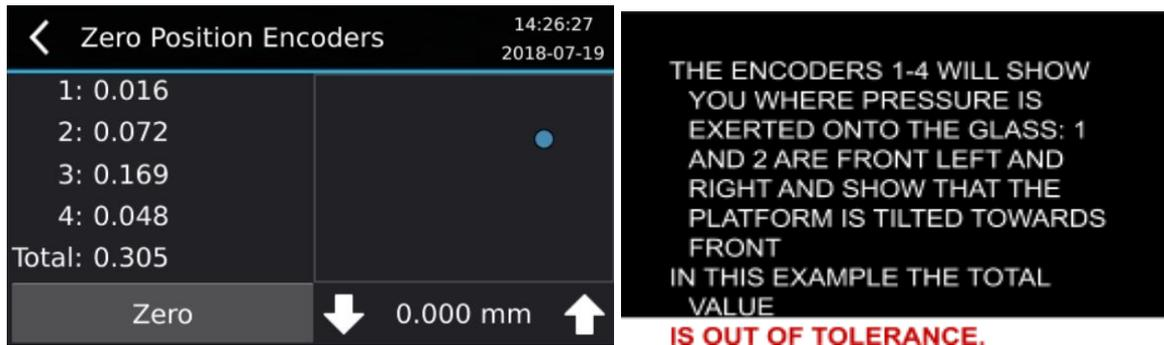
**If the total value is out of range, e.g. showing 0.100 or greater, this will lead to Approach fails or traversed layers.** In this instance part of the platform at zero position is touching the glass and the target position for the first layer will not be reached
